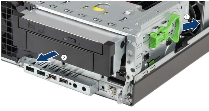
Figure 47: Removing the 5.25-inch ODD/HDD bracket
